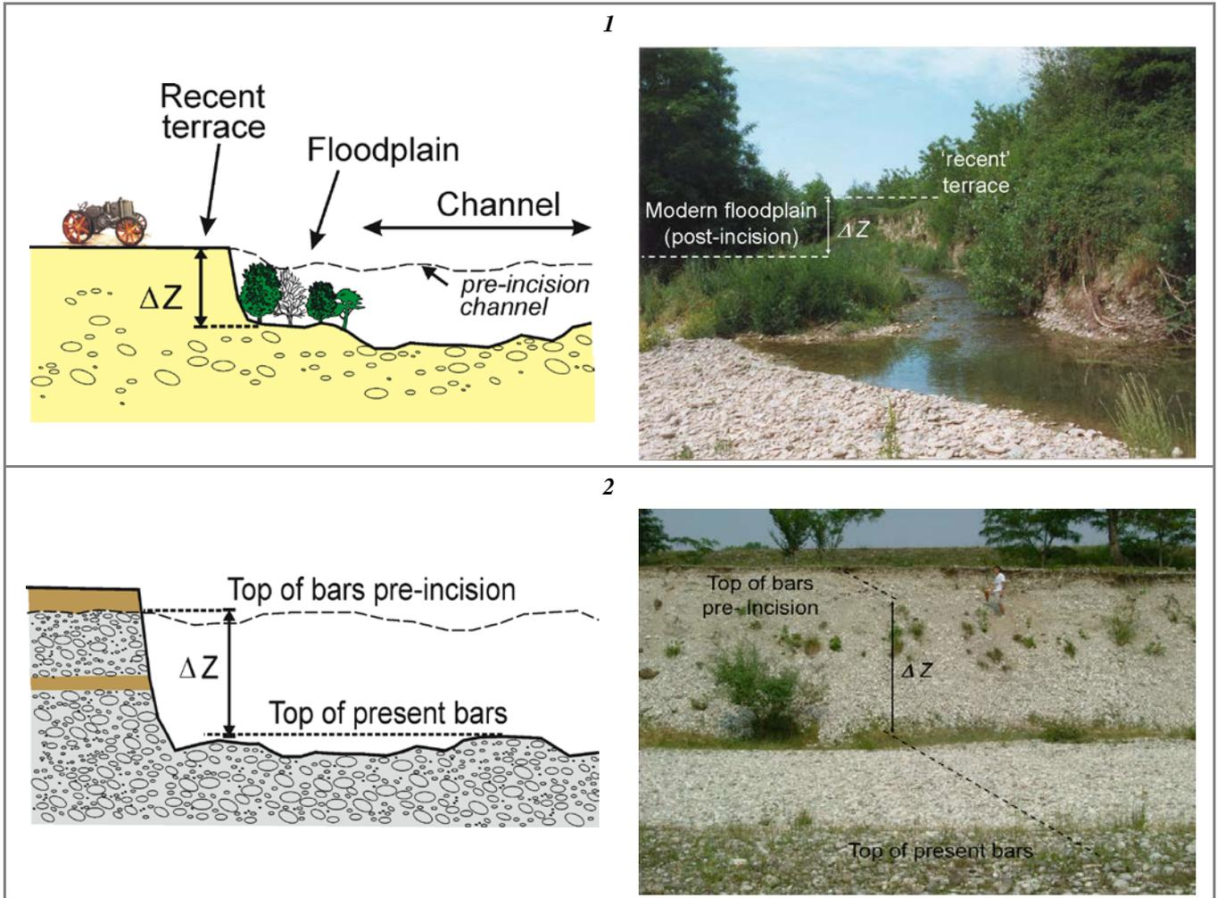
**Figure 82** – Estimation of the amount of incision based on differences in elevation among surfaces. (1) Measurement of difference in elevation ( $\Delta Z$ ) between modern floodplain and recent terrace (pre- incision floodplain); (2) measurement of difference in elevation between the top of gravel on an eroding bank (corresponding to the top of bars before incision) and top of present channel bars.
