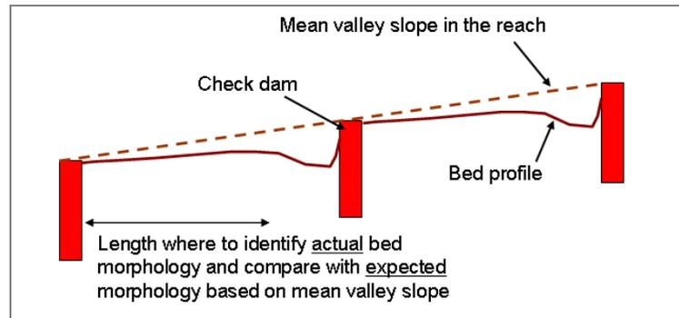
**Figure 34** – Bed configuration and valley slope. Rule for the measurement of the mean valley slope of the reach in the presence of structures (check dams) and to identify the length of analysis of bed morphology.
