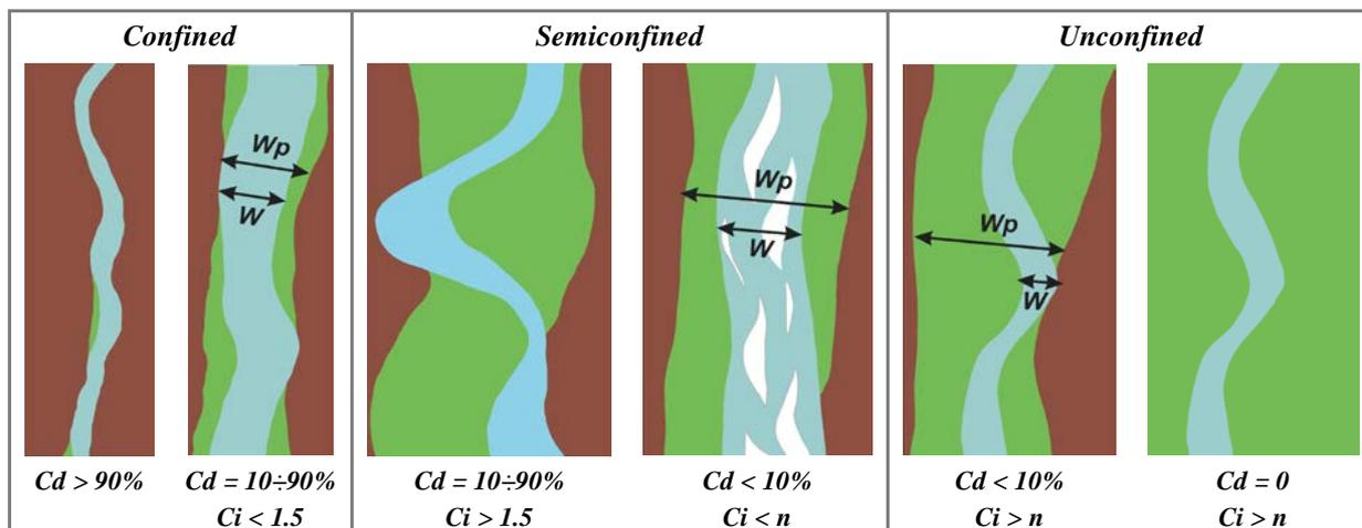
**Figure 3** – Confinement classes. In green: alluvial plain; in brown: hillslopes (or ancient terraces).  $Cd$ : confinement degree;  $Ci$ : confinement index =  $Wp/W$ , where  $Wp$ : alluvial plain width (including the channel) and  $W$ : channel width.
