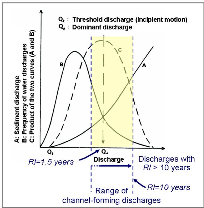
**Figure 53** – Range of channel-forming discharges, including the discharges with return interval of up to 10 years.  $Q_{1.5}$  (discharge with a return interval of 1.5 years) is the value conventionally assumed as the most representative of channel-forming discharges.
