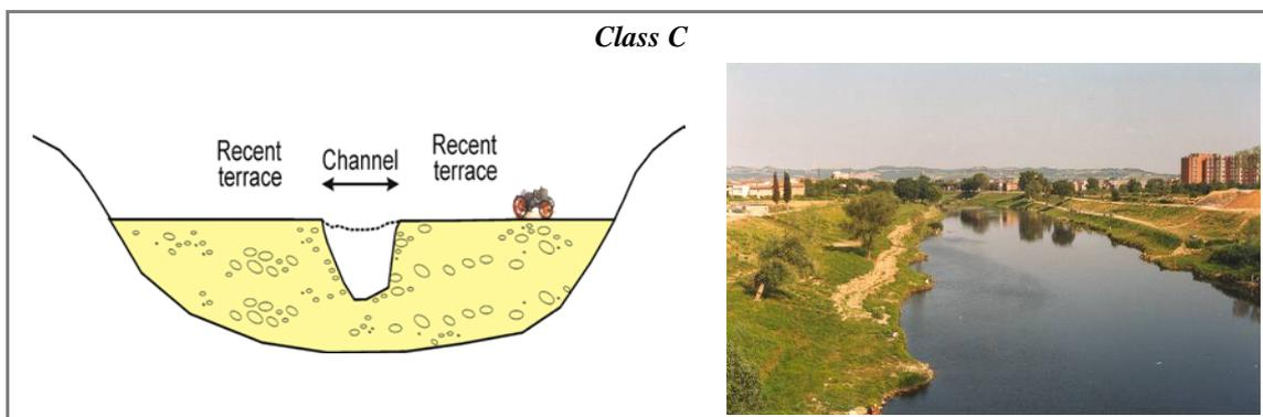
**Figure 30** – CASE 6: the channel is heavily incised ( $> 6$  m) and vegetation corridor that could be a post-incision floodplain is absent (*F12* in *Class C*), therefore the reach is necessarily in *Class C*.
